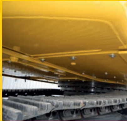
Heavy duty undercovers (9 mm) fully enclose the upper structure's underside for enhanced protection against debris on the ground.
